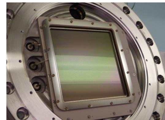
Figure 21: INFUSE (2023) 100 mm XS Detector with 25 μm resels.
