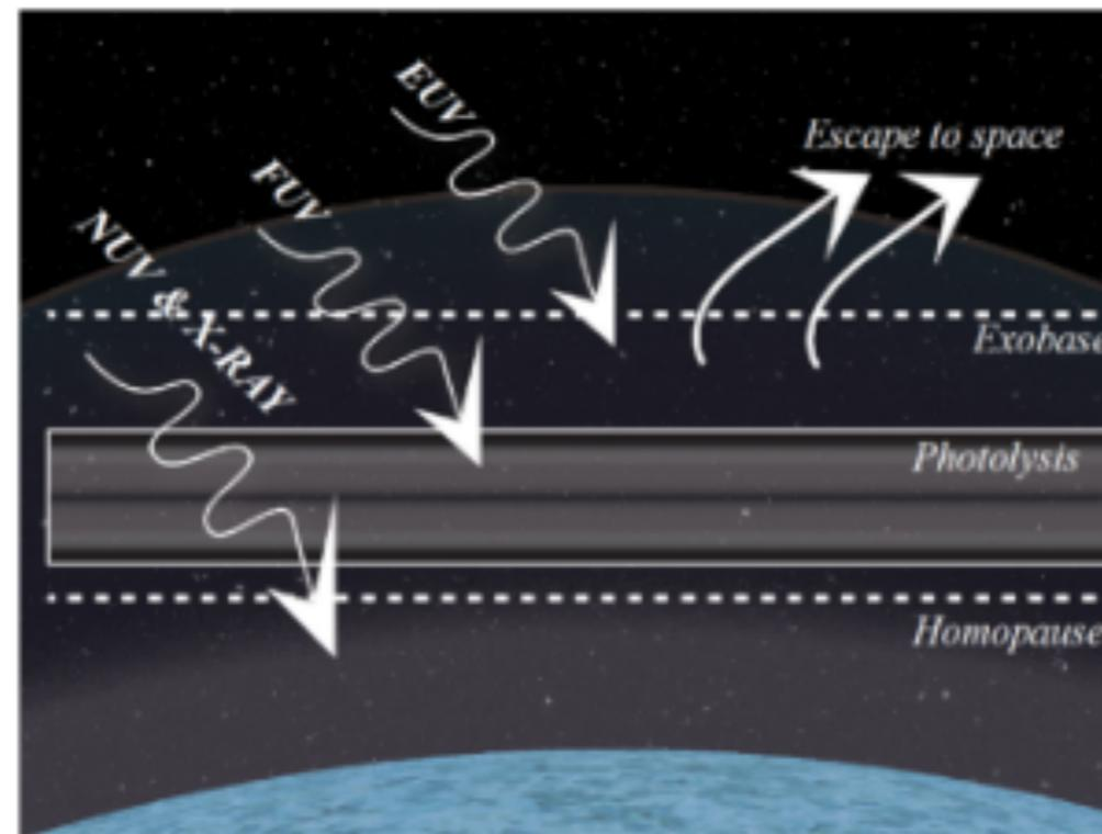
**Figure 1:** The ultraviolet stellar spectrum drives photochemistry (FUV and NUV photons, 100 – 320 nm) and atmospheric escape (EUV photons, 10 – 90 nm) on orbiting planets. The EUV spectrum is calculated from chromospheric and coronal lines in the FUV spectrum, with the 100 – 115 nm band providing unique diagnostics for temperature and abundances. The host star spectra are used to predict the most promising habitable planet candidates and to interpret atmospheric spectra (Tsai et al. 2023).
