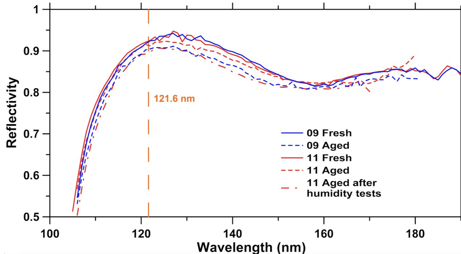
**Figure 35:** Reflectivity of two XeLiF samples (ID 09 and 11) both fresh and aged (18 and 12 weeks, respectively).
