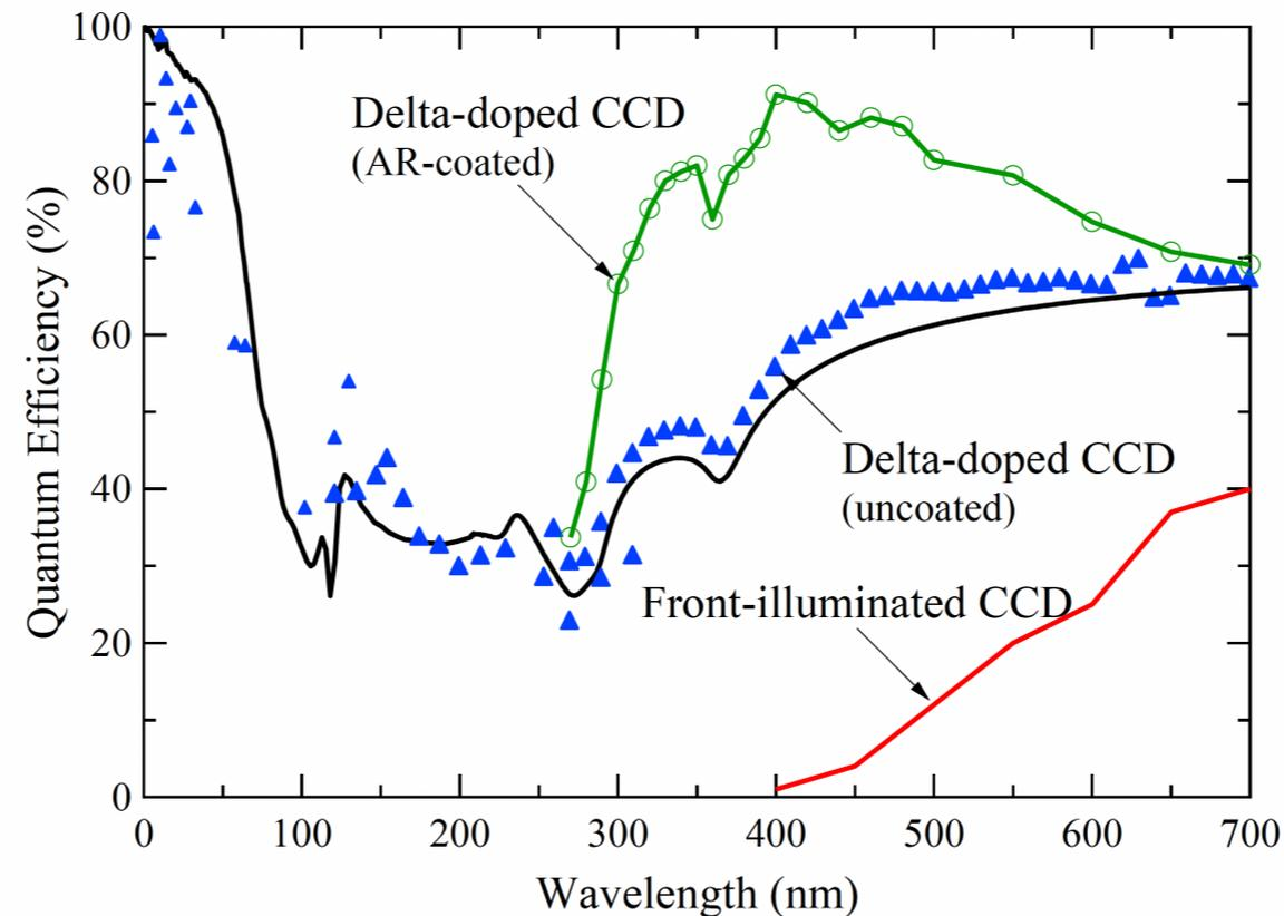
**Figure 23:** Delta-doping involves a doping layer to a back-illuminated silicon detector, which eliminates an electron well in the detector surface. The result is silicon detectors sensitive in the UV. The QE can be further increased by the addition of anti-reflection coatings. In the figures, solid lines are models, markers are measurements (Hoenk et al. 2022).
