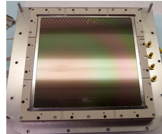
Figure 20: 20 x 20 cm Microchannel Plate with XDL readout for the DUCE rocket program.
